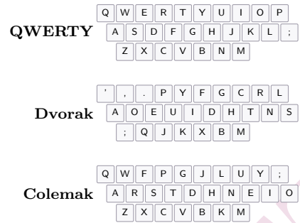
Figure 2: Three typing keymaps over the same physical substrate. Each layout is a re-binding of identical key positions to a different set of letters. QWERTY (Sholes 1873, never patented), Dvorak (Dvorak & Dealey 1936, US 2,040,248), Colemak (Coleman 2006, public domain). The post-2010 fork ecosystem extends this line.
